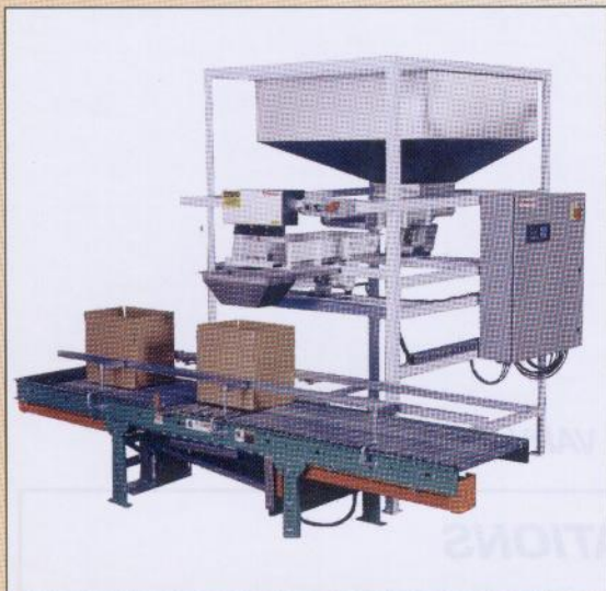
Direct Fill System with Automatic Container Indexing System
